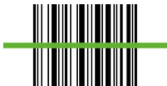
PowerScan™ PBT9100 provides an aiming system. If enabled, a partial trigger press produces a flashing scan line, which should be aimed over the code, see figure above. By completely pressing the trigger the scan line becomes continuous to start the code scanning.
