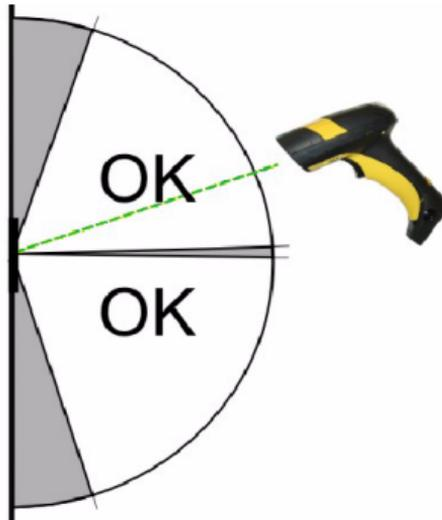
Symbologies with smaller bars or elements (mil size) should be read closer to the unit. Symbologies with larger bars or elements (mil size) should be read farther from the unit.
