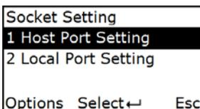
Step 8: Press Scan/Select Key to bond with the target host. "🔗" indicate the connecting process.
