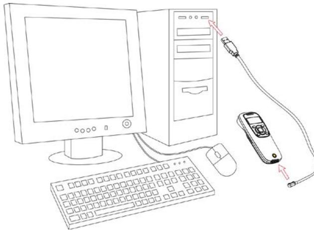
**Figure 2-1 Diagram of connecting the terminal to PC**
