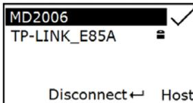
Step 7: Press Right-Soft Key to display the **Host Lists Menu**. In **Host Lists Menu**, press the navigational key to select the target host IP. The screen shows as follow:
