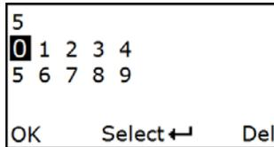
Step 3: Use Navigation Keys to move the cursor, Scan/Select Key to select number(s), Right Soft Key to delete selected number(s). And then press Left Soft Key to continue.
