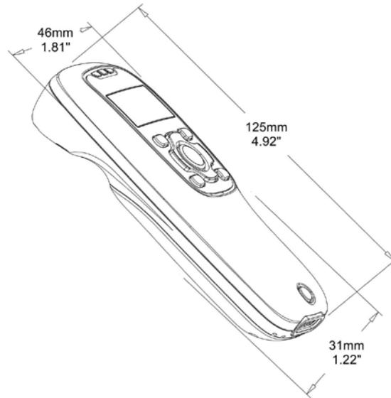
**Figure 1-1 Dimensions of the terminal**
