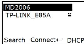
Step 4: Press the Right-Soft Key to enter the DHCP setting menu, press the navigational key to select whether enable DHCP, and press the Scan/Select Key to confirm. If disable the DHCP, you should input the static address for the terminal. The screen shows as follow:
